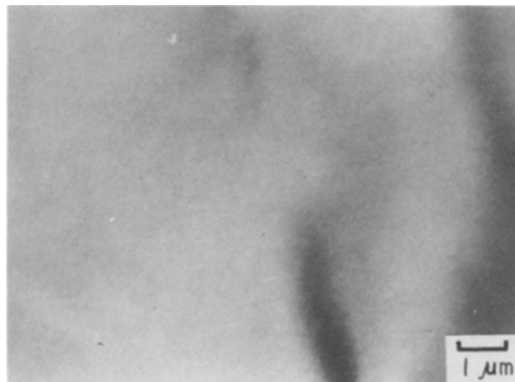
Figure 2 Electron micrograph of GaP diffused with Zn and P sources at 850° C for 1 hr. Zn: 0.2 \text{ mg cm}^{-3} ; P: 0.05 \text{ mg cm}^{-3} .
